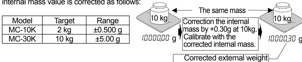
Step 1 Calibrate the balance using the internal mass. (one-touch calibration).
