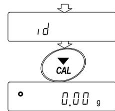
Step 11 Press the **CAL** key to calibrate the balance using the internal mass.
