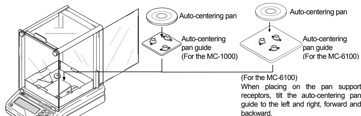
**Note: When replacing the weighing pan with the auto-centering pan, be sure to calibrate the balance before weighing, because the two pans are different in weight.**
