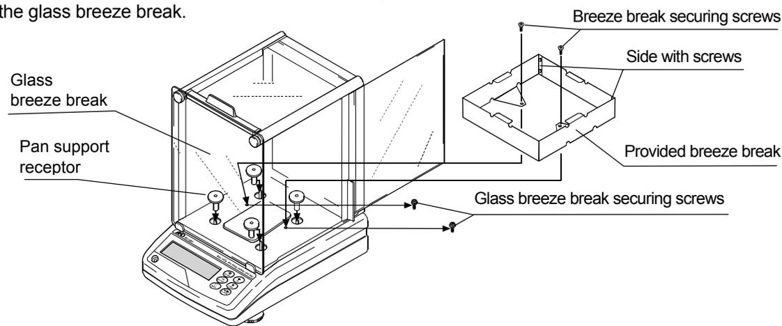
2. Place the auto-centering pan guide on the pan support receptors, and then place the auto-centering pan on the guide.
